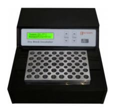
The block is made of an aluminum alloy with excellent thermal conductivity and has different hole sizes for 1.5 & 0.5 ml microtubes..
