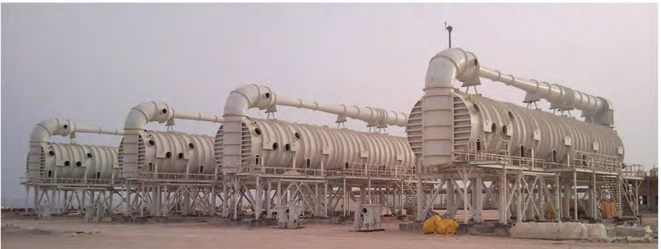
Complete Design of four 4000 m 3 /day MED-TVC Units – South Pars Gas Field, Phases 15 & 16
