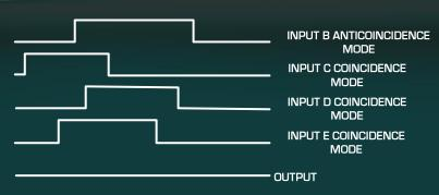
Coincidence Requirements When Switch Setting is 3.
