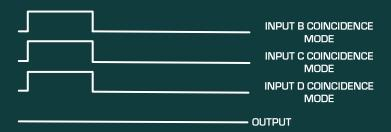
Coincidence Requirements When Switch Setting is 4.
