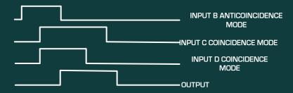
Coincidence Requirements When Switch Setting is 2.
