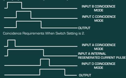
Coincidence Requirements When Switch Setting is 2.
