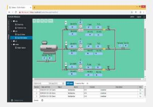
The user is able to select a view (table or schema) and the date of access to the archive data. To display the input channel diagram, the user just have to click on a the related icon in a table or a suitable element in a layout. WebStation is available from any computer or tablet connected to the organization's network without the need to install special software. The access to the views and the controls is managed by the admin system, which determines the level of user access.
