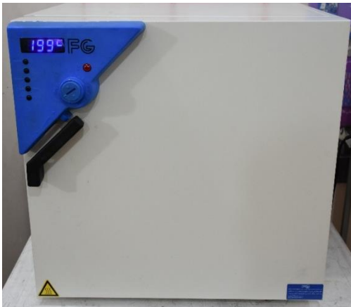
Laboratory Oven up to 200 °C
