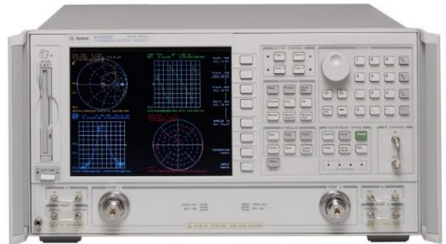
8720E Agilent Network Analyzer 20GHz
