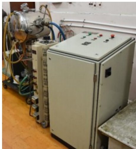
Induction furnace in vacuum (5 KW)
