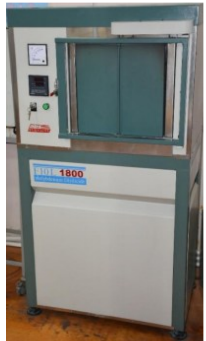
Oxidation furnace up to 1700 °C
