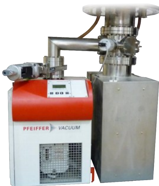
Vacuum System (Turbo Molecular & Ion Pumps)
