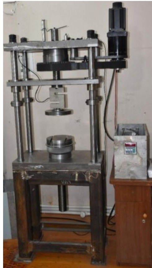
Uniaxial die-press up to 15 ton with servo motor control
