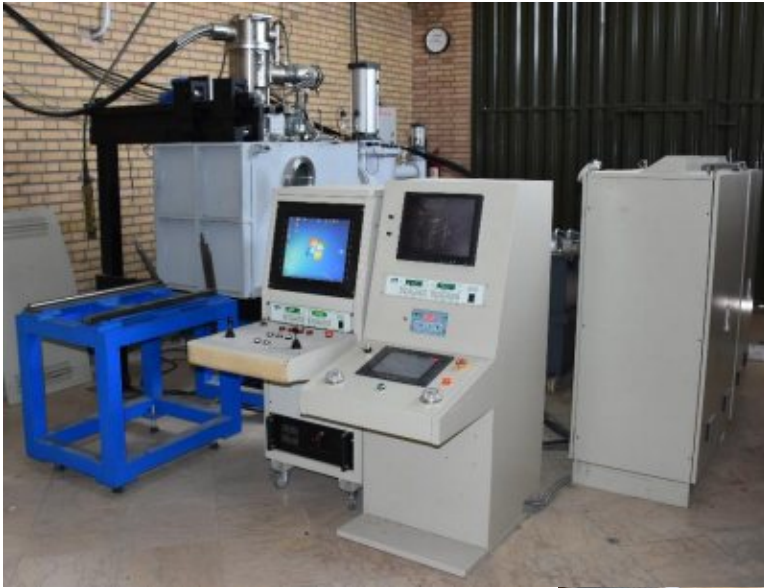
85 kV , 235 mA Electron beam power
