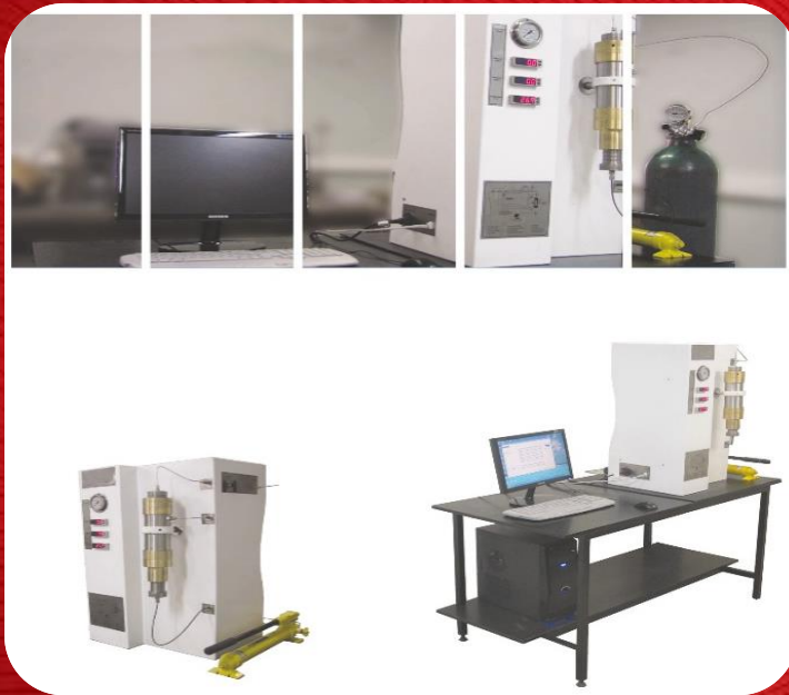
Unsteady State Gas Permeameter
