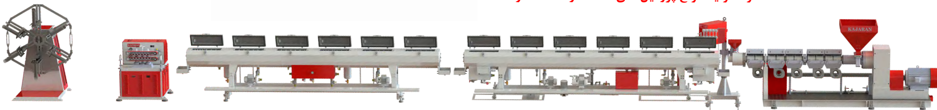
PE ,PP, PVC Pipes Production Line
