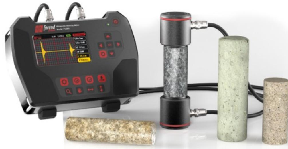
Ultrasonic Pulse Velocity Meter
