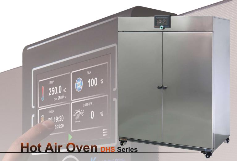
The Oven or Dry Heat Sterilization (DHS) is an electrical furnace that uses for drying, sterilization and depyrogen processes by creating heat in a chamber. This device is used in laboratories and production lines of pharmaceutical industry, medical diagnostic laboratories, research and development laboratories of biological products.
