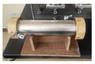
remains inside the core holder; the core is loaded from one end without the need of filling/draining the confining fluid. By releasing the confining radial and axial pressures and unscrewing the end plug, the core sample can easily be removed without exposure to the hydraulic fluid. The core holder can be configured for Hassler, Hydrostatic or Triaxial loading.
