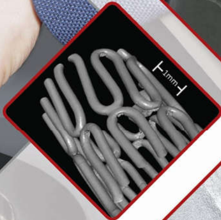
Coronary stent imaged by LOTUS-NDT micro-CT.
