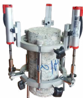
ELP50-3 The exact longitudinal strain (For Compression) Double Sensor
