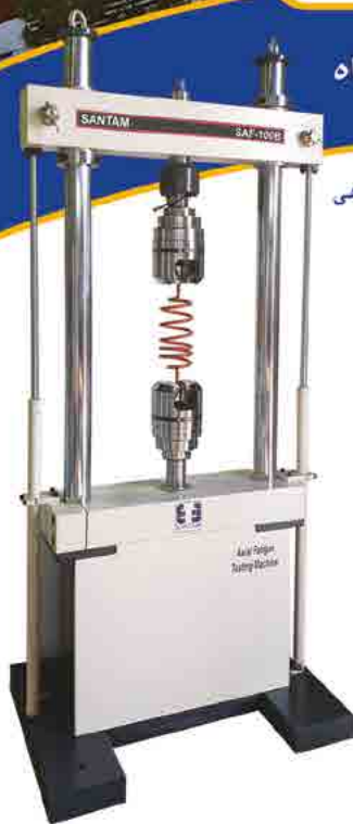
Axial Fatigue Testing Machine High response servo hydraulic SAF-100B 100 kN Capacity
