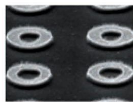
FESEM Images of Micro and Nano Structures Etched by DRIE(SI-HV300)
