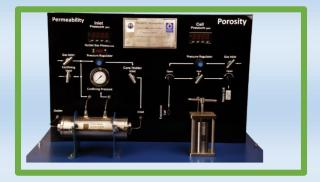
GasPerm can be operated in standalone mode of remotely through the optional PC interface. An excel report ready-to-use is provided. The operator (or the software) writes the data and the permeability is calculated automatically.
