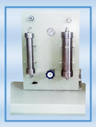
The GOR apparatus features the capability of recirculating the evolved gas back through the on board high pressure oil pycnometer and gas pycnometer. This recirculation ensures liquid vapor equilibrium and allows the operator easy representative homogeneous access to samples of atmospheric pressure vapor and liquids. The establishment of equilibrium is essential for high pressure volatile liquids such as those encountered in reservoir fluid studies.
